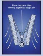
thereby preventing excessive wear due to disc "flutter."
